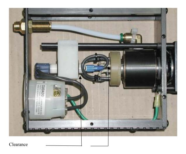
View of slip ring wiring. Next picture is with HS shaft rotated 90 degrees.
